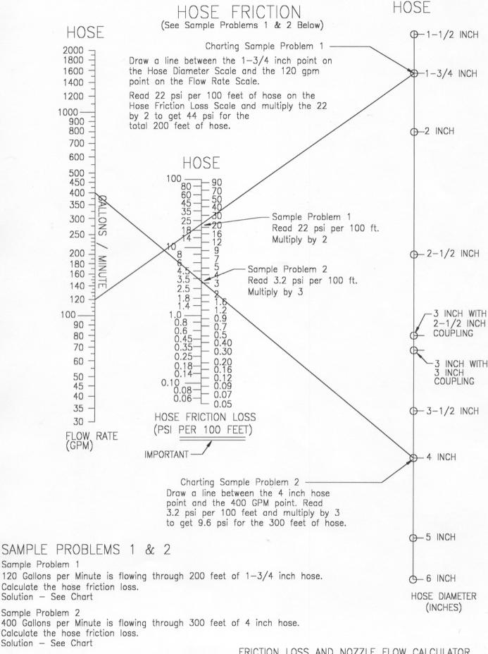
FRICTION LOSS AND NOZZLE FLOW CALCULATOR
